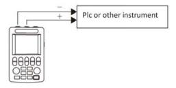
output active current/voltage to instrument
