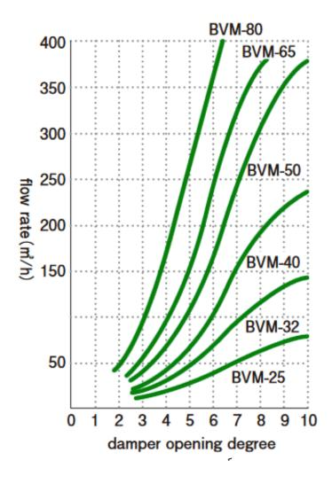
**BVM flow characteristics** when differential pressure  $\triangle P = 1.5 \text{ kPa}.$
