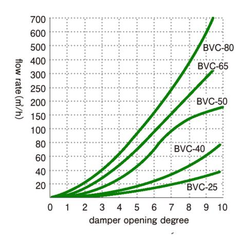
**BVC flow characteristics** when differential pressure  $\Delta P = 1.0 \text{ kPa}.$
